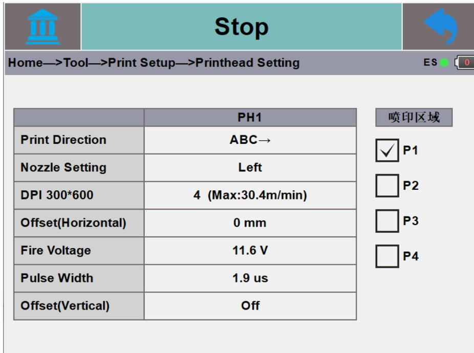
You can change the printing direction according to the running direction of the production line by this interface
