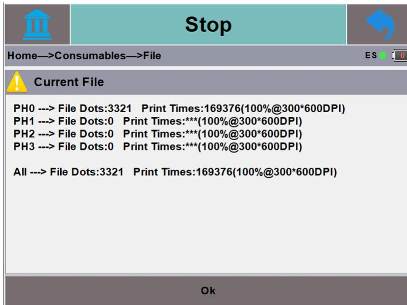
You can see the ink volume information and the current printing time from this interface. When printing starts, the system will automatically calculate the approximate usable time. Users can decide the inventory of ink cartridge based on this information to prevent the shortage of ink cartridges from affecting production.
