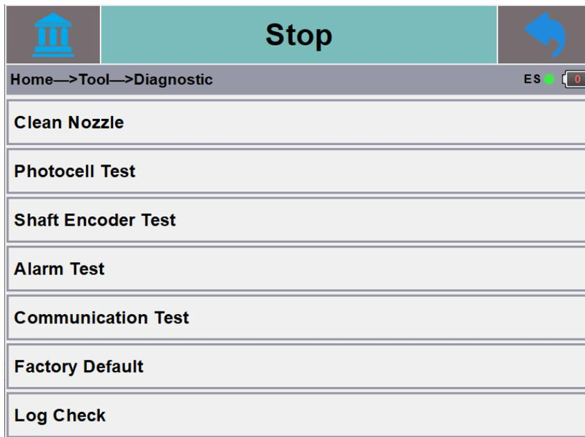
When the machine fails, you can rectify the general fault according to the system prompts in this menu. If the machine still cannot be used normally after troubleshooting, please contact your equipment supplier or manufacturer.
