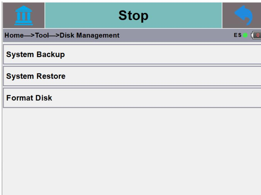
Users can use U disk to back up machine data and parameters, or restore previous backup information or parameters, and format the disk.
