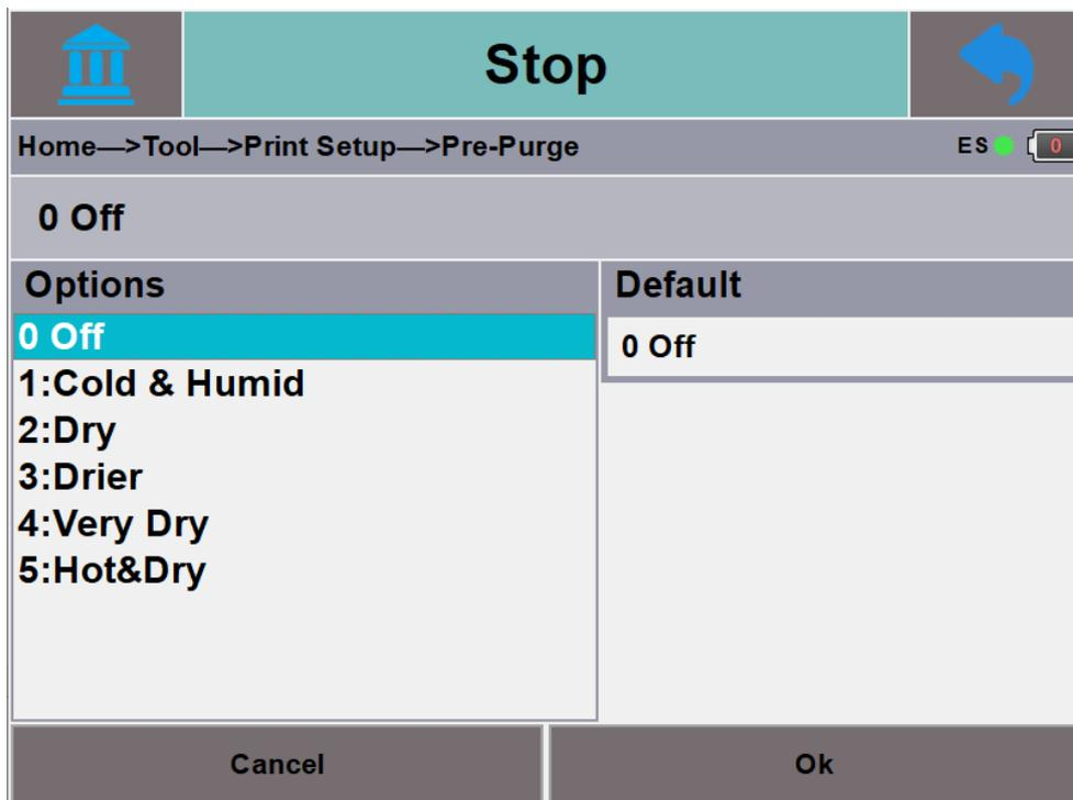
When the printing interval is longer and the air is relatively dry, the printing effect may be affected. In order to overcome this problem, the system will pre-flush the nozzles according to the ambient air level set in this menu to improve the printing effect.
