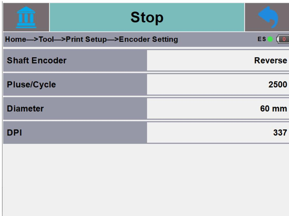
When the encoder is set to "forward or reverse", the pulse number (PPR) and the diameter of the encoder wheel (mm) should be input according to the parameters, and the system will calculate the width of the printing information accordingly, the width will not change with the change of production speed.
