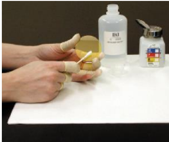
Figure 7-3 focus mirror moderate pollution cleaning
